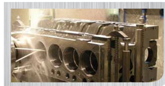
Fully automatic engine block machining
