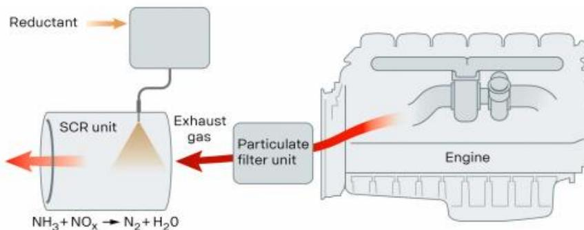
A chemical process is started when reductant, a urea and water mixture, is injected into the exhaust gas stream. During injection, the water evaporates and the urea breaks down to form ammonia. The ammonia then reacts with the nitrogen oxide gases in the catalytic converter and forms harmless products such as nitrogen gas and water.
